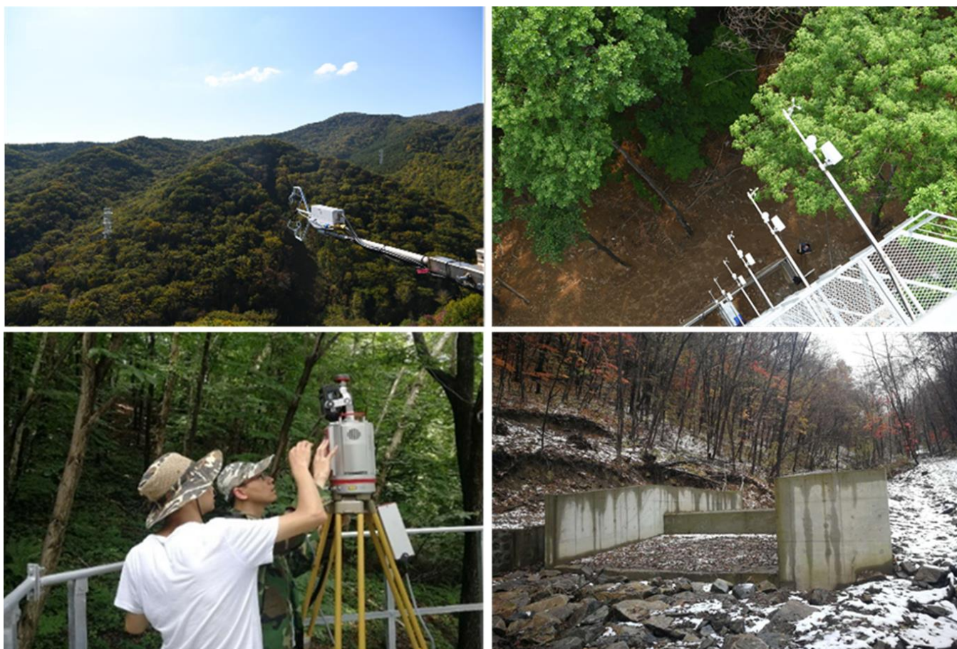
Fig. 4 Long-term measurement systems: Closed-path eddy-covariance flux measurement system (CPEC310, top-left), atmospheric profile system (AP200, top-right), tower-based LiDAR scanning operation (bottom-left), and watershed hydrology station (bottom-right).
