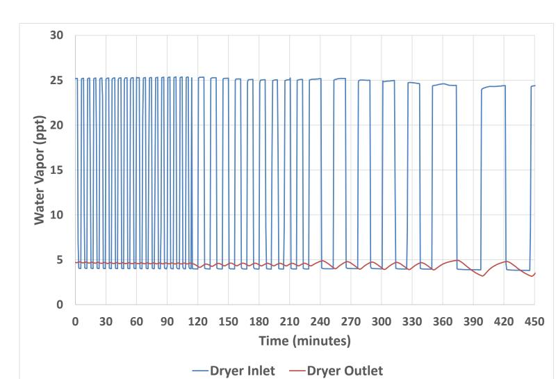
function was calculated as the ratio: dryer outlet/dryer inlet.
