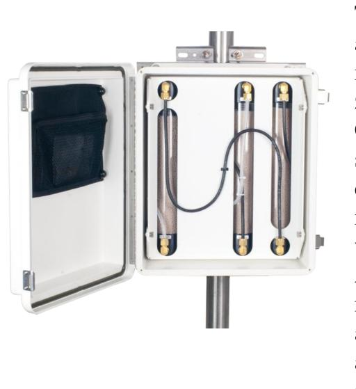
The CPEC200 Scrub Module is an accessory to the CPEC200. It is used to provide a source of zero air for zeroing the EC155  $CO_2/H_2O$  analyzer. It uses a small, low-power (2W) diaphragm pump that is mounted in a temperature-controlled and weathertight fiberglass enclosure Ambient air is drawn through molecular sieve to remove  $CO_2$ and water vapor, and push zero air to the EC155 at approximately 2 l·min<sup>-1</sup> flow.
