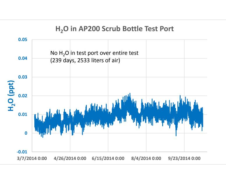
The AP200 Scrub Bottle will easily last a year in normal operation. The test port gives an indication it is time to replace the molecular sieve with a large safety margin.
