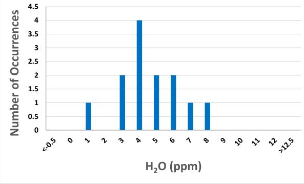
All cylinders tested at  $CO_2 < 0.3$  ppm; below specifications. Water vapor was between 0 and 8 ppm, but still well below practical requirements for an IRGA intended for ambient humidity. In all cases the zero air had equal or less CO<sub>2</sub> and H<sub>2</sub>O after passing through the molecular sieve.
