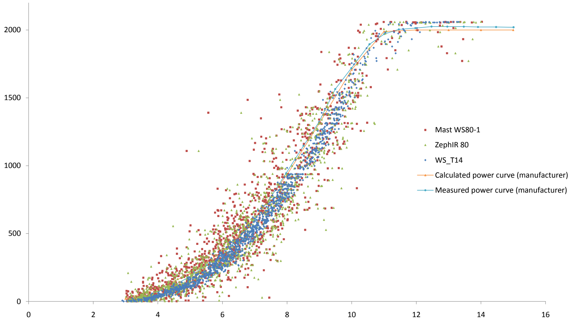
Figure B-10 Power produced by turbine 14 against mean wind speed measured with nacelle anemometer, the mast (WS80-1) and ZephIR at 80 m
