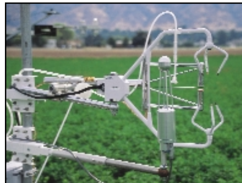
The CS7500 (front), with a CSAT3 (middle), and KH20 (rear), makes measurements in an eddy covariance application.
