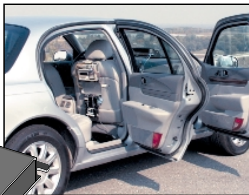
A test vehicle (above) stands instrumented with sensors, datalogger, Heads-Up Display and peripherals. The DCDC18R (left) is a compact package designed to attach to the side of a CR23X or CR5000 rechargeable base.
