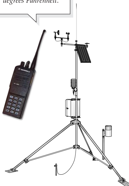
The VSP3 Vosponder allows hand-held UHF or VHF radios to call monitoring stations and receive a verbal report of data.
