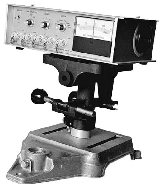
The CA9 Path Averaging Laser Anemometer was the first engineering product at Campbell Scientific.
