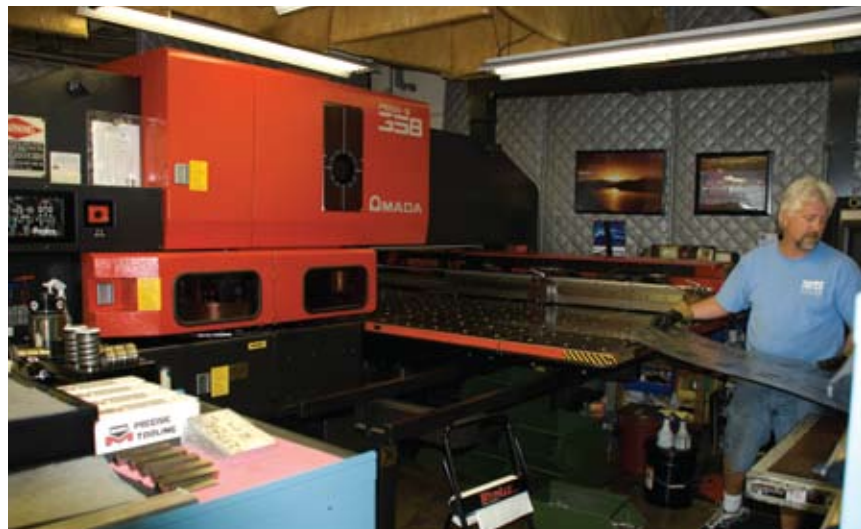
Our numerically controlled pick-and-place machine (left) is used to manufacture printed-circuit assemblies. The numerically controlled multi-station turret punch (right) is used to manufacture precision sheet-metal chassis and mounts.
