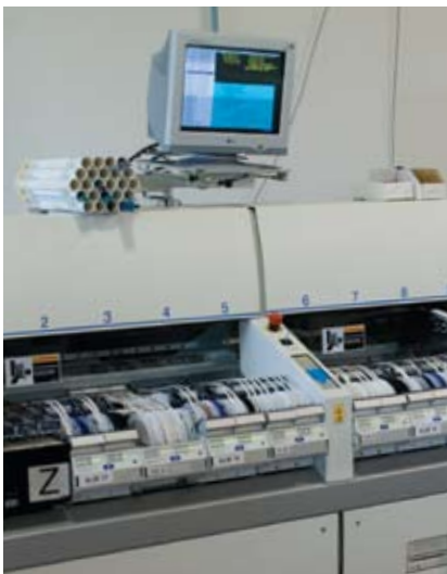
Our numerically controlled pick-and-place machine (left) is used to manufacture printed-circuit assemblies. The numerically controlled multi-station turret punch (right) is used to manufacture precision sheet-metal chassis and mounts.
