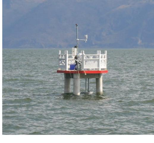
atmospheric pressure, and precipitation with a single instrument. To measure dissolved oxygen, pH, algae, and conductivity in the water, Beijing Techno Solutions chose an MS5 sonde from Hydrolab with several sensors bundled together in one product.
