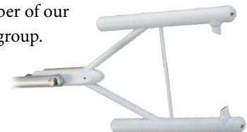
The EC150 measures trace gases as they pass through the measurement space.
