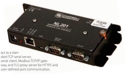
By providing both simple Ethernet communications and complex networking capabilities, the NL201 is a powerful device that can meet your networking needs in a wide range of applications.
