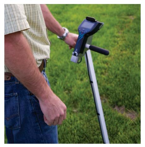
The HS2P HydroSense II Pole, Campbell Scientific's newest HydroSense soil-water measurement product, facilitates both the insertion of the probe into the soil and its removal. The HS2P has an aluminum insertion pole that is lightweight, yet sturdy enough to handle repeated soil insertions and removals. Because the pole is used
