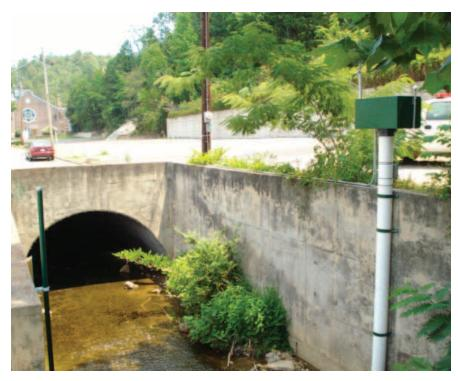
Four of the stations report stream stage and rainfall. Each station contains a CR1000 datalogger, NL120 Ethernet interface, COM320 voice-synthesizing telephone modem, and GOES satellite transmitter. Measurements are reported via the Internet and the GOES system. Alarms are delivered directly from the station via text and interactive phone messaging.
