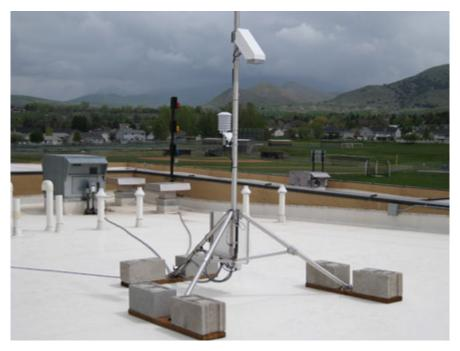
second alarm every two minutes, warns that there is enough electric charge in the atmosphere to trigger a lightning strike.
