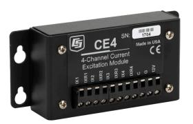
The number of 229 sensors measured by one datalogger can be increased by connecting a CE4 or CE8 to one or more AM16/32-series multiplexers<sup>2</sup>. Up to four multiplexers can be connected to the CE4, and up to eight multiplexers can be connected to the CE8.
