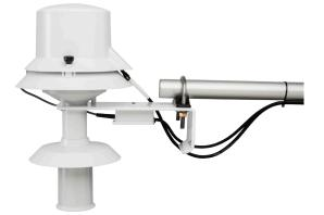
For the 2 m measurement, the 43502 attaches to the legs of a UT20 or UT30 tower via a CM202, CM203, CM204, or CM206 crossarm. Two CM210s can be used to attach the crossarm to two tower legs.
