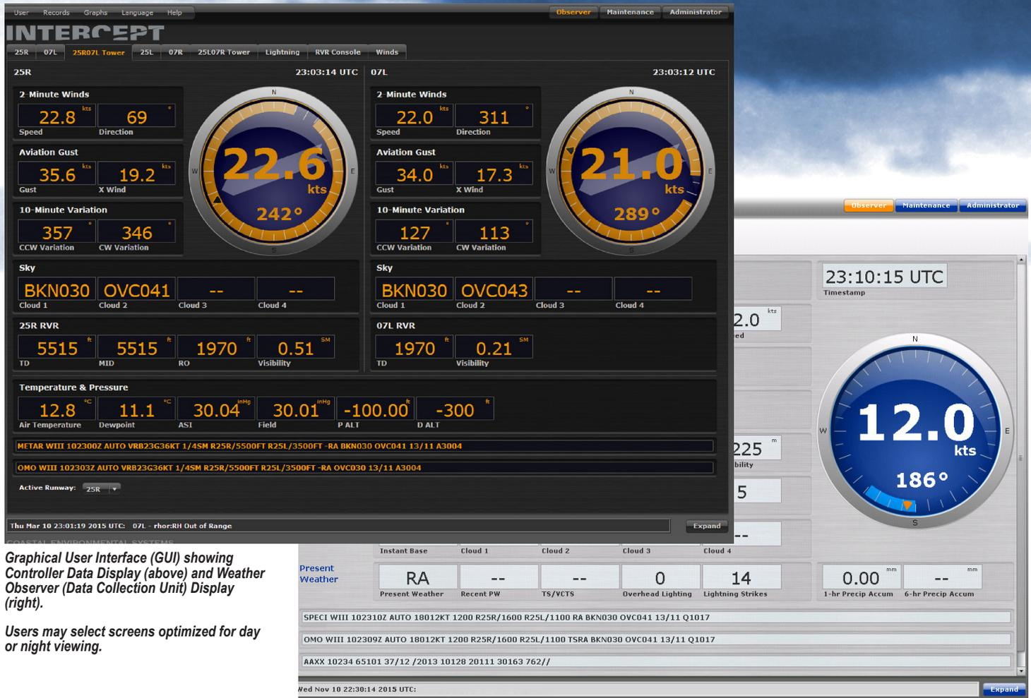
Graphical User Interface (GUI) showing Controller Data Display (above) and Weather Observer (Data Collection Unit) Display (right).
