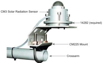
To attach the CM225 to a CM202, CM204, or CM206 crossarm, place the u-bolt in the holes on the bottom of the bracket (shown). If the CM225 is attached to a mast, place the u-bolt in the holes in the side of the bracket.
