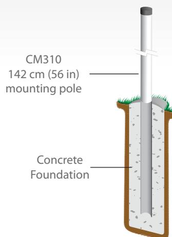
This cut away view shows a 142 cm (56 in) mounting pole placed directly in a concrete foundation. Order a CM310-NP to get a 142 cm (56 in) pole without a pedestal kit.
