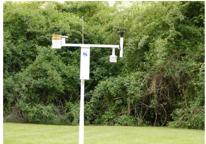
The ET107 is an automated ETo station for commercial agriculture, irrigation scheduling, and meteorological applications
