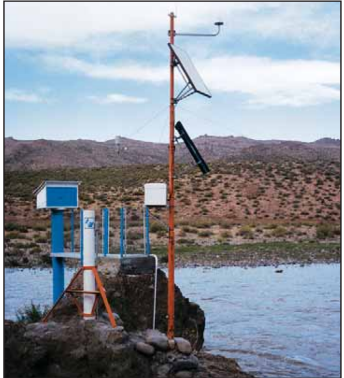
A satellite transmitter provides telecommunications for remote Argentine stations where phone lines are impractical.
