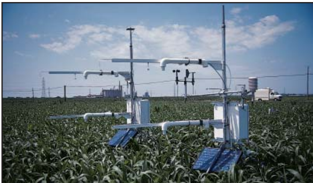
Bowen Ratio Systems calculate evapotranspiration and CO 2 fluxes over a sorghum field near Lincoln, Nebraska.
