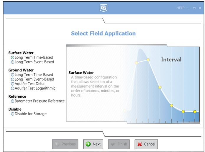
HydroSci software is included with the CRS451V/CRS456V. It simplifies the process of configuring the sensor to monitor surface water, ground water, or a standard pump test.
