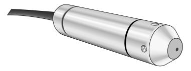
Each transducer is shipped with a calibration sheet. The sheet specifies I/O conditions, as well as actual data reflecting the unit's static accuracy and thermal characteristics. Each vented transducer is also shipped with a desiccant tube to extract water vapor from air entering the vent tube.
