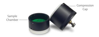
Soil is placed in the sample chamber and compacted to a chosen pressure by using the compression cap.
