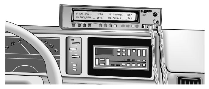
The DSP4 is a real-time data display for use with Campbell Scientific dataloggers in vehicle testing applications. The DSP4's low-profile packaging permits dashboard mounting in a variety of vehicles without obstructing the driver's view. The DSP4 displays four measurements with user-defined labels and input ID numbers. Selection of displayed measurements can be changed quickly with push-button switches.
