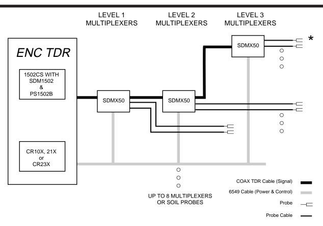
★ For rock-mass deformation applications, the soil probe sensors are replaced with user-supplied coaxial cables.
