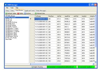
The Data Review tab shows tables and data from the database. When a table on the left side is selected, the data for the table is shown on the right side.
