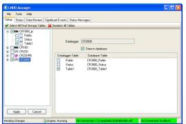
When a station is highlighted in the left tree, the station setup screen is shown. On the station setup screen, tables can be enabled/disabled for storage.
