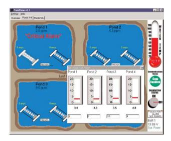
To quickly check dissolved oxygen levels and alarm conditions in all ponds, PondView provides an overview page. Up to six groups of six ponds can be displayed — allowing you to easily monitor what is happening in each of 36 ponds.
