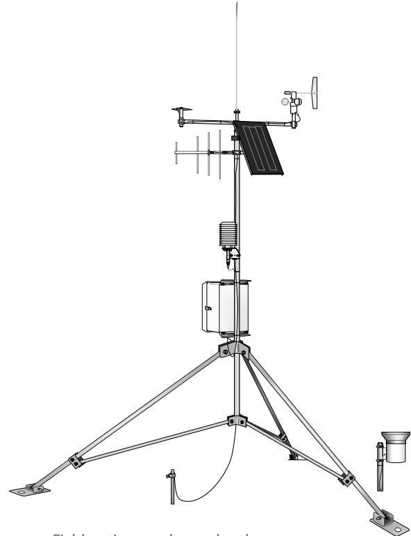
Field stations are located at the measurement site. This field station uses a Yagi antenna to transmit the data.
