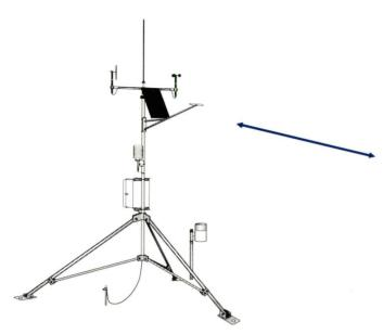
Sensor measurement, data processing/storage, and on-site control functions are performed by a CR10T datalogger. The CR10T features the same measurement and control hardware as the CR10, but contains table-oriented final data storage, which provides more efficient data transfer through modems to the RTMS computer.
