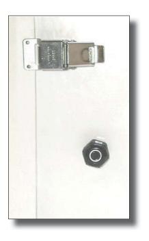
At left is a closeup of the SC-IRDA Interface mounted in an enclosure compression fitting. To communicate with the datalogger, point the PDA's IRDA sensor at the SC-IRDA sensor head exposed on the outside of the enclosure.
