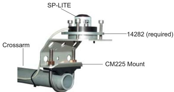
*To attach the CM225 to a horizontal crossarm, place the u-bolt in the holes on the bottom of the bracket (shown). To attach the CM225 to a vertical mast or pole, place the u-bolt in the holes in the side of the bracket.*
