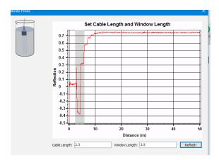
PCTDR 3.0 has a calibration wizard that helps users quickly determine the appropriate cable length and window length.
