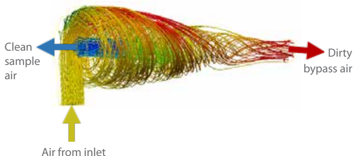
Figure 1. Streamline flows through the vortex. Warmer colors represent higher speeds of dirty air to the right (towards bypass), and cooler colors represent higher speeds of clean air to the left (towards sample cell).
