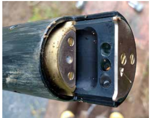
Figure 3B. OBS501 with shutter open during a maintenance visit
