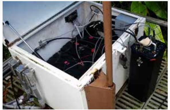
Figure 2B. Campbell Scientific custom datalogger enclosure designed to meet WET specifications
