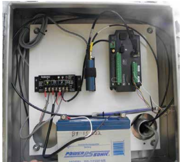
Figure 1. Campbell Scientific datalogger, pressure transducer, battery, solar charging system, cellular digital modem
