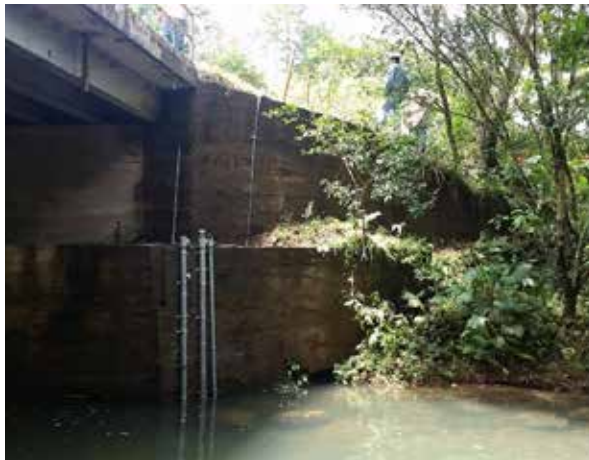
Figure 3A. Conduit for the turbidity and conductivity and temperature sensors as well as the sampler hose
