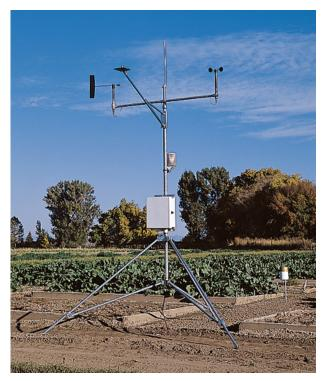
Many researchers place a weather station adjacent to test plots for a continuous record of meteorological conditions that could impact their research.
