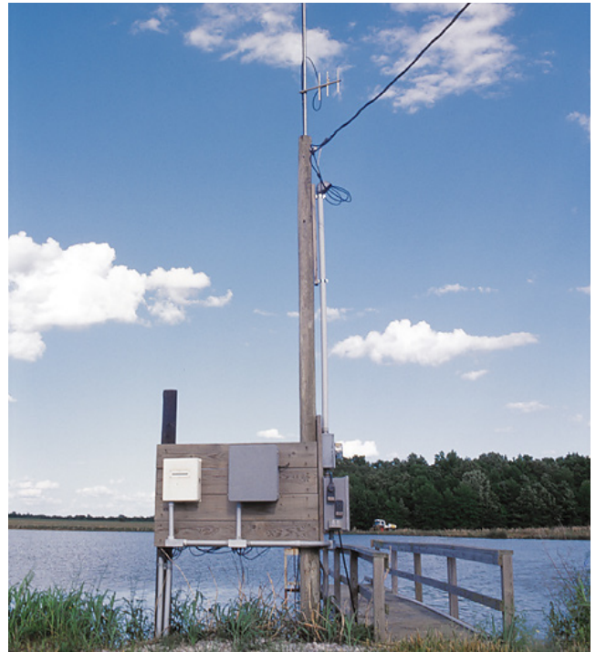
For Lee's catfish farm in Mississippi, our equipment eliminated the need to manually check dissolved oxygen concentrations.
