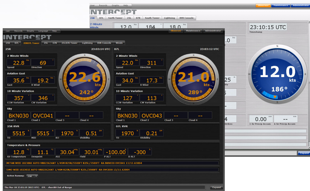
Graphical User Interface (GUI) showing Controller Data Display (above) and Weather Observer (Data Collection Unit) Display (right). Users may select screens optimized for day or night viewing.
