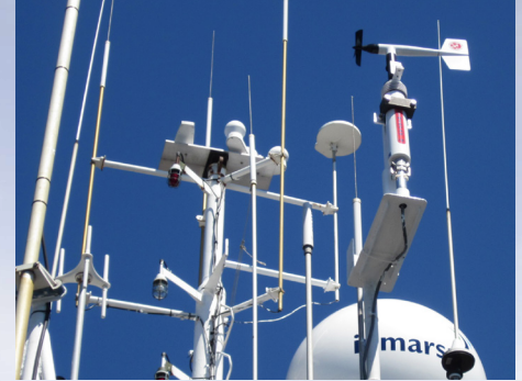
Single point WEATHERPAK® system on a research vessel
