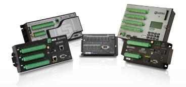
The control functions of our dataloggers allow them to sound alarms and control devices based on time or measured conditions.
