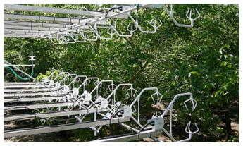
The California walnut groves's sensor arrays provided a large data set used to confirm models linking turbulence and elements of weather, climate, and plant growth.
