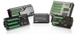
Our dataloggers also feature programmable scan rates, measurement types, and recording intervals and provide onboard statistical and mathematical functions for on-site data management.
