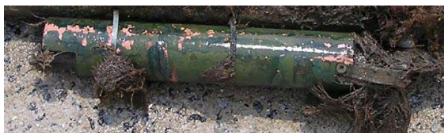
Figure 19. Copper sleeve after 137 days at Skidaway Georgia site
