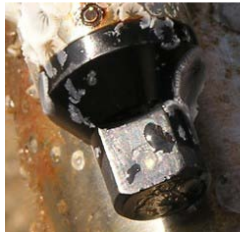
Figure 8. Baseline sensor, day 36 after manual cleaning
