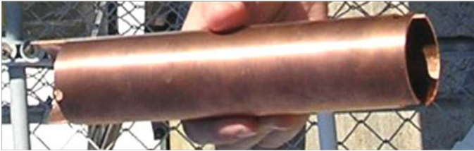
Figure 5. Copper sleeve to prevent fouling of sensor body
