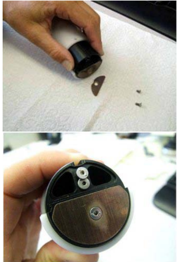
Figure 4. Refillable biocide chamber
