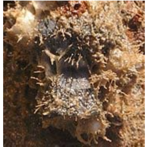
Figure 7. Baseline sensor, day 36 before cleaning
