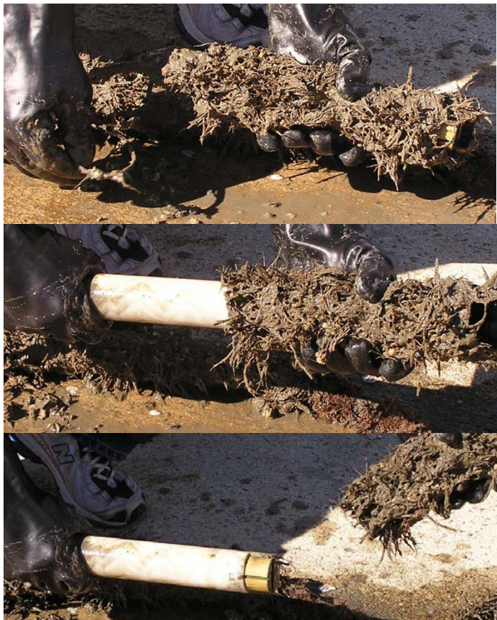
Figure 17. Process of removing a disposable plastic sleeve
