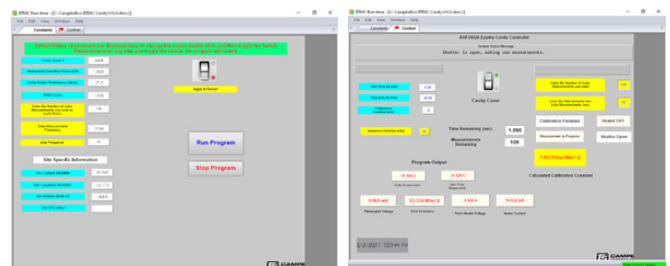
Figure 3. Screenshots of the RTMC Run-time control screens. The first is the initial setup screen. The second is the main display used during operation. Note that the irradiance is directly displayed to the user.
