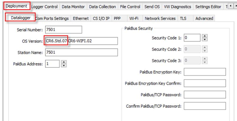
11. Check to see what version of the WiFi daughter board operating system your datalogger is running. As in the previous step, you can see this information in the **Deployment | Datalogger** tab in *DevConfig*. The **OS Version** field shows the datalogger operating system version and WiFi daughter board operating system version (in red below) currently loaded into the datalogger.
