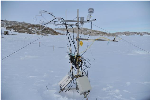
**Figure 2.** The eddy-covariance station located in the coastal landfast sea ice area of Antarctica Zhongshan Station ( $69^{\circ}22' \text{ S}$ ,  $76^{\circ}22' \text{ E}$ ). It was configured with the IRGASON integrated  $\text{CO}_2/\text{H}_2\text{O}$  open-path gas analyzer and three-dimensional sonic anemometer, CNR4 four-component net radiometer, HMP155A air temperature and relative humidity probe, and SI-111 infrared radiometer.
