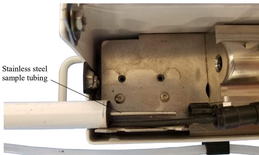
**Step 12:** Remove the stainless steel sample tubing by gently pulling it from the outer tube.
