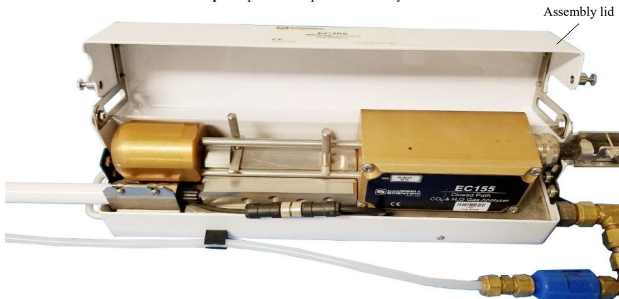
**Step 4:** Loosen the thumbscrews and position the latches so the struts of the analyzer are free.
