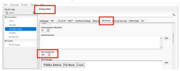
To change the setting in *LoggerNet* select your data logger on the **Setup** screen. On the **Hardware** tab set the **Maximum Packet Size** to **200**.
