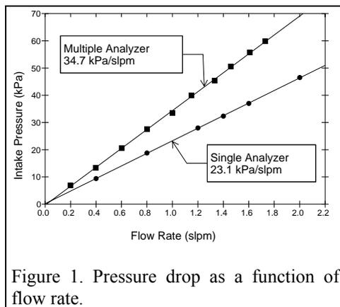
Figure 1. Pressure drop as a function of flow rate.
