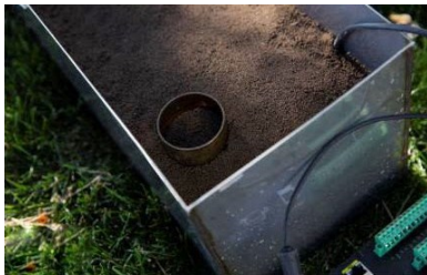
FIGURE 3-4. Ring placed in trough next to rods
