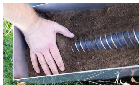
FIGURE 3-2. Packing soil around the SoilVUE™10
