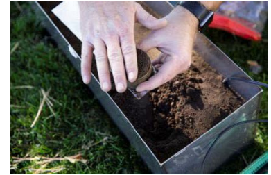
FIGURE 3-7. Lifting ring out of soil
